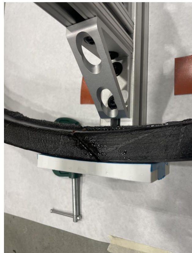
Bond lines appear larger than 0.05 mm, could be due to bonding jig inaccuracies
