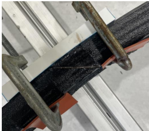
Bonded scarf joints with Araldite 2011 mixed with microballoons (to ensure 0.05 mm bond line)
