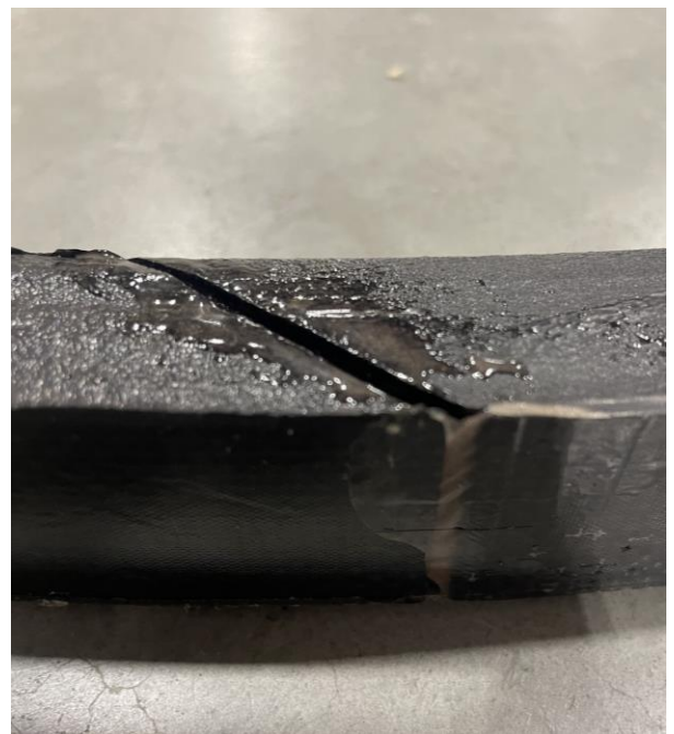
Bonded joints show some adhesive sag on top face (area to machine still has full adhesive coverage)
