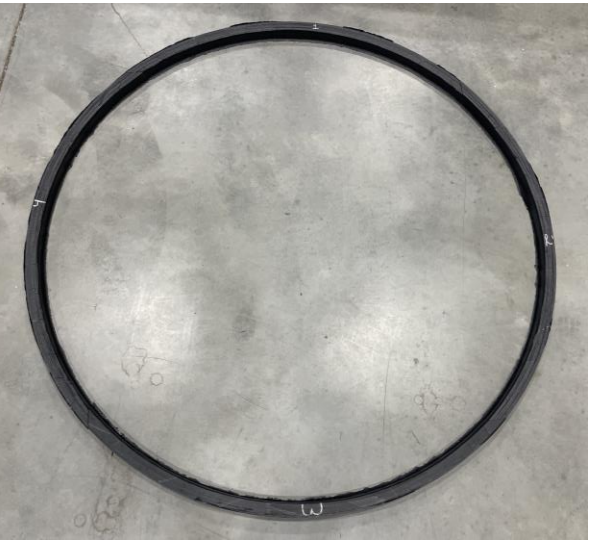
Assembled end ring (~0.05 mm bond line)
