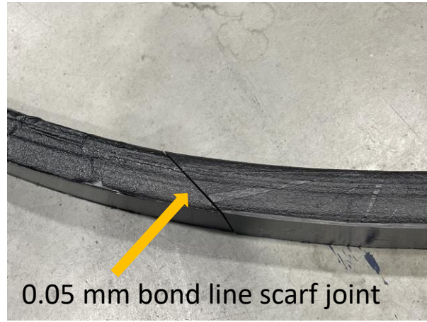
Machined scarf joint on both sides, accounting for 0.05 mm adhesive bond line thickness
