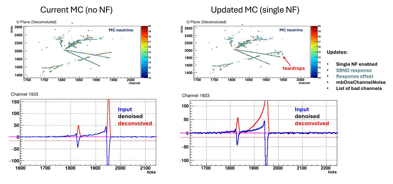
Signal is protected after noise filtering in both cases. Deconvolved waveform (red) with noise filtering shows a positive porch not seen in deconvolved waveform without NF. What could be causing the creation of that porch?
