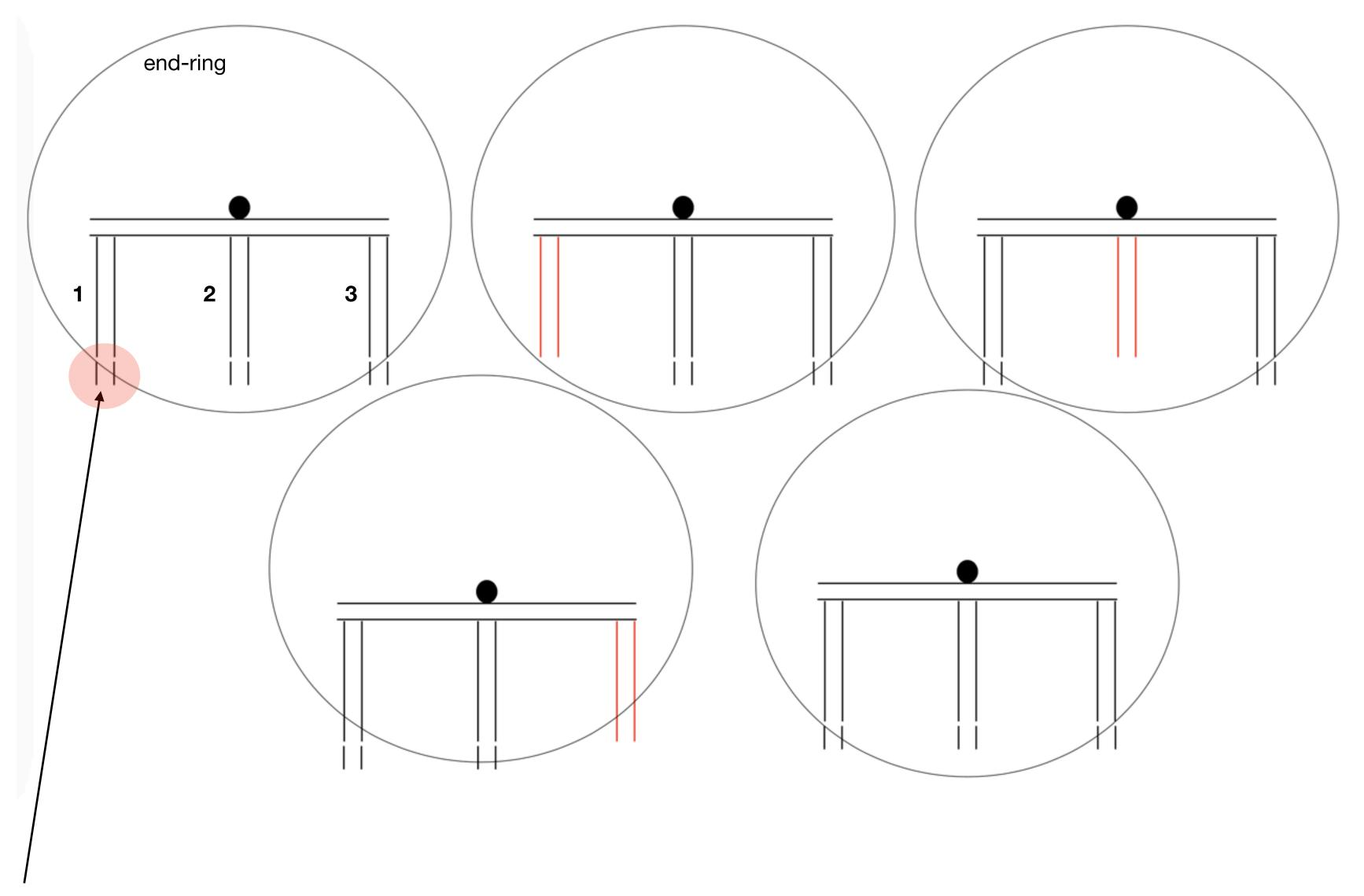
The lower part of each leg can be removed. Combine 1, 2, and 3 for the installation.
