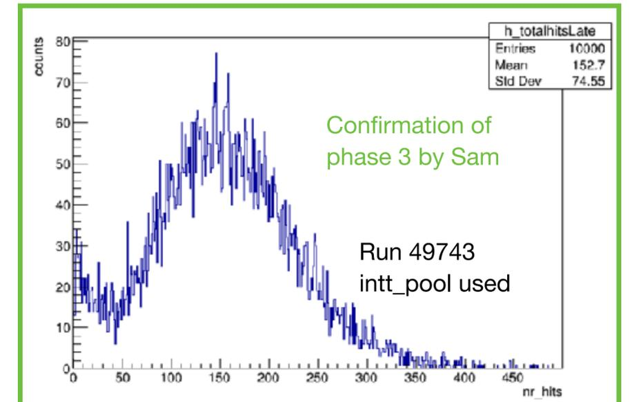
Total hits rate(?) of data at the beginning of file and after skipping 700k RCDAQ events. Data of phase 3 looks consistent with that of phase 1.
