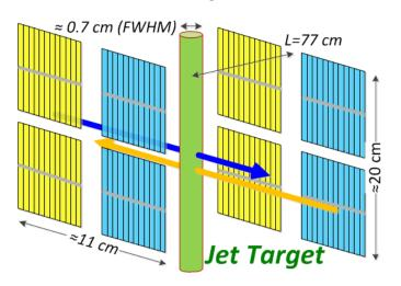
Asymmetry of the recoil proton detection is measured for the beam and target (the jet) spins simultaneously and in the same Si detectors:
