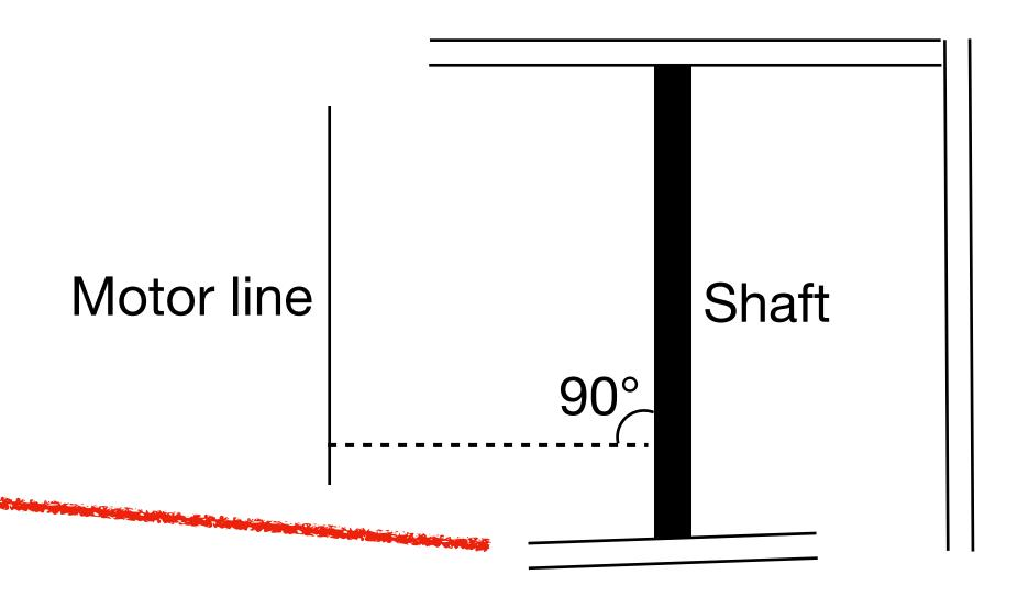
The shaft is aligned with the motor line
