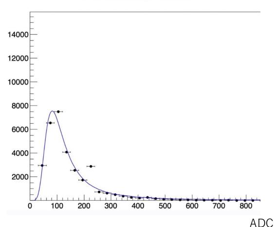
I learned the fitting method by using a convolution function of Landau and Gaussian, and I could run the program.
