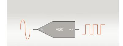
ADC is Analog Digital Converter
