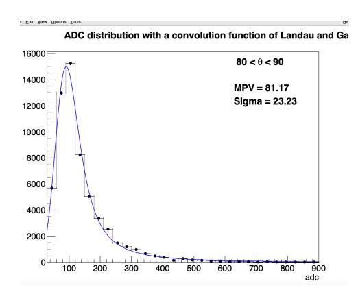
Though I could not determine yet how much of an effect the noise has, I added new fitting method by using a convolution function of Landau and Gaussian
