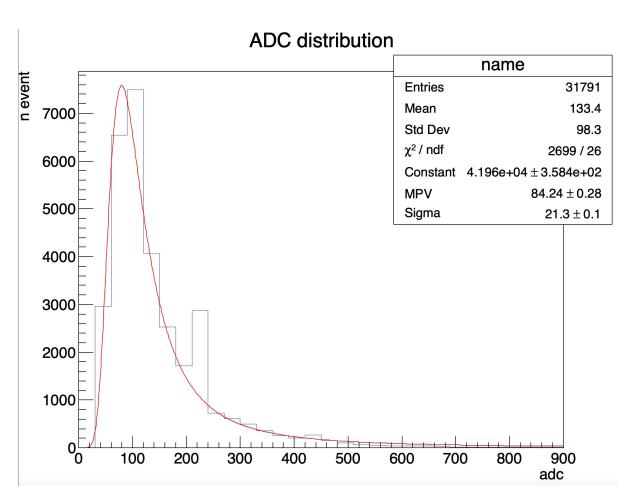
The plot on the left is the MIP peak by applying a cut of the tracking  $\theta$  to the ADC distribution.
