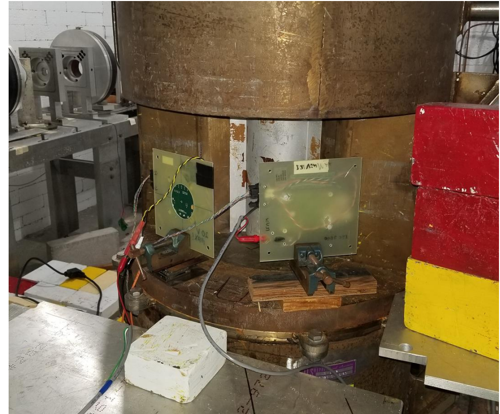
Two devices are tested at a time with both receiving the same dose
