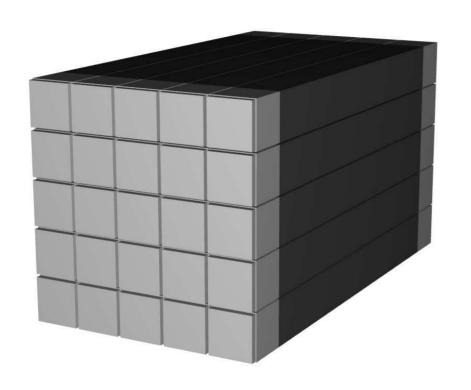
HomogeneousCalorimeter\_geo.cpp and backward\_PbWO4.xml have been modified to place modules in a matrix
