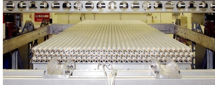
Muon MDT chamber, tube d=3 cm, 80μm/wire
