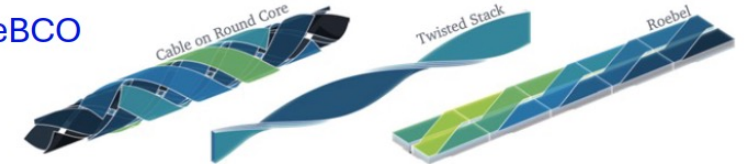
Figure 1.10. Three different geometries for assembling a cable with ReBCO coated conductor. Also refer to Table 1.2.
