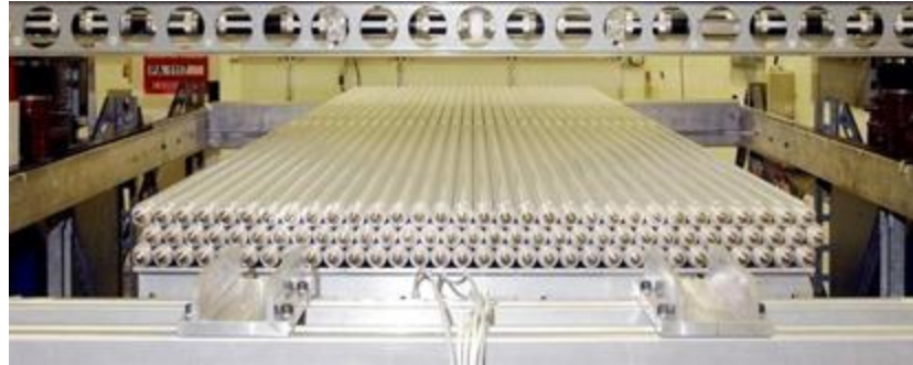
Muon MDT chamber, tube d=3 cm, 80\mu\text{m}/\text{wire}
