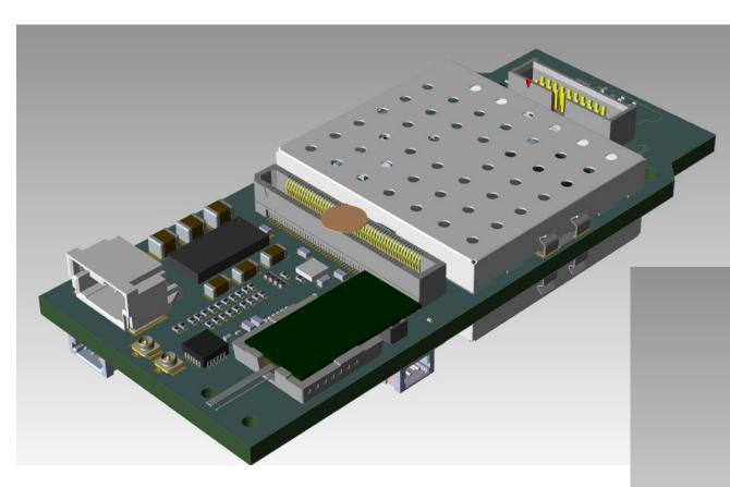
layout modified to allow possibility to mount cages (over FPGA) to shield EMI emission (to be tested real effectiveness/need but layout allows for that)
