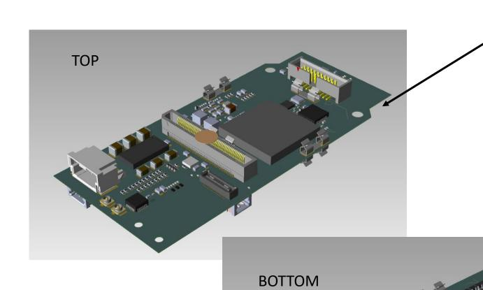
modified shape to allow space in dRICH PDU of cooling cables
