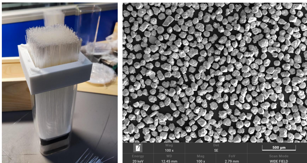
Figure 8.92: Matrix of scintillating fibers prepared to build production fEMCal blocks and SEM image of tungsten powder.
