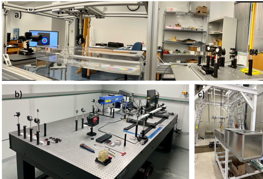
Figure 8.51: Photos of available setups developed during the hpDIRC R&D program that will be used for future QA of 3-layer lenses with laser setup at ODU (a), bars and other optics at Jefferson Lab (b) and readout chain including sensors and electronics and other hpDIRC components in hpDIRC prototype at CRT at SBU (c).
