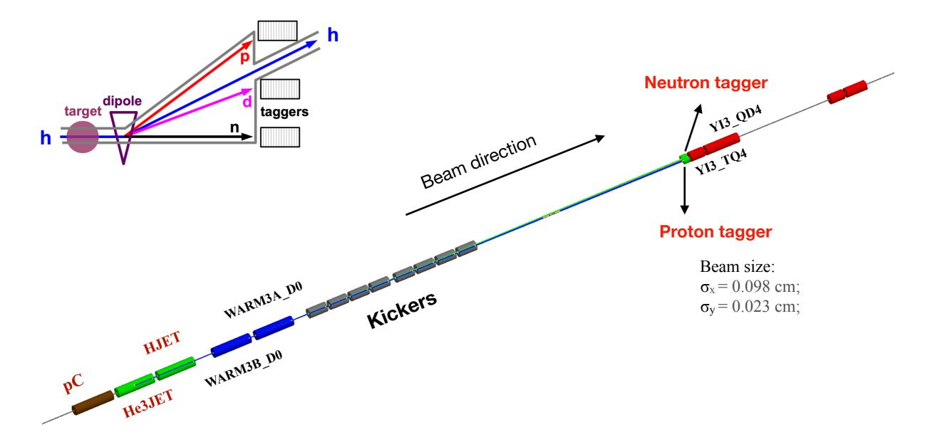
• Proposed placement of Stochastic Cooling Kickers between the He3JET and the tagger.
