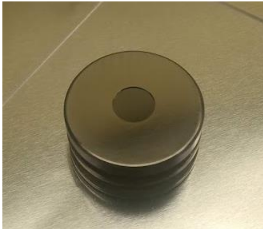
The modified CeC Mo cathode puck with a square GaAs crystal inserted under a metal cup with a 5 mm hole in diameter.
