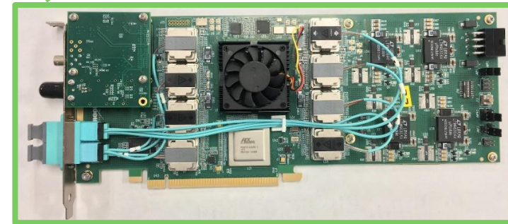
Global Timing Module (NSLS II/sPHENIX) Receiving from RHIC RF low jitter clock source
