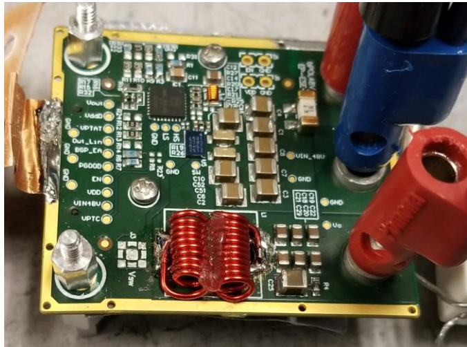
bPOL48V w/ bottom mount heat-sink, 300nH @ 1.5MHz Inductor dimensions: 10 x 12.0 x 7.5mm (LxWxH)
