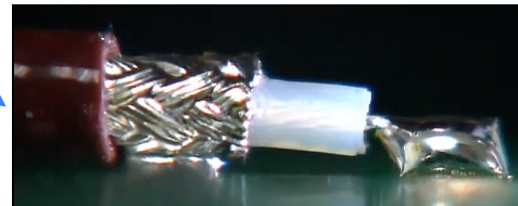
HV Coax cable soldered to pad Teledyne PN: 167-2896 26AWG
