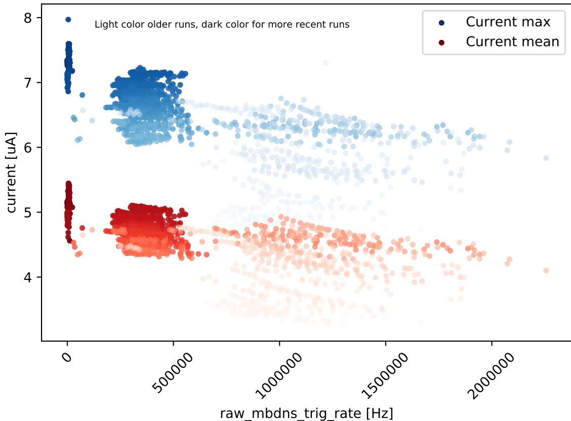
INTT RC-0S, duration > 10.00 min, trigger_rate vs. sensor current
