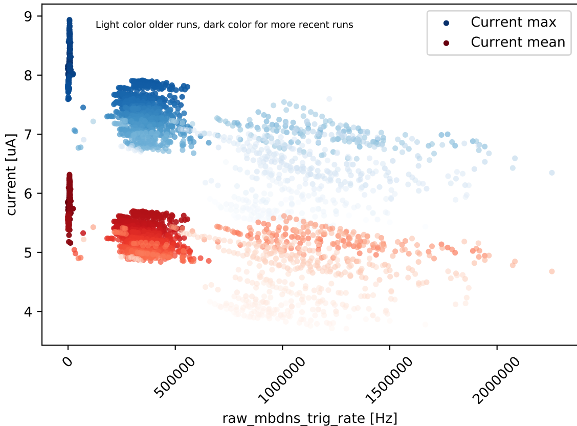
INTT RC-5S, duration > 10.00 min, trigger_rate vs. sensor current
