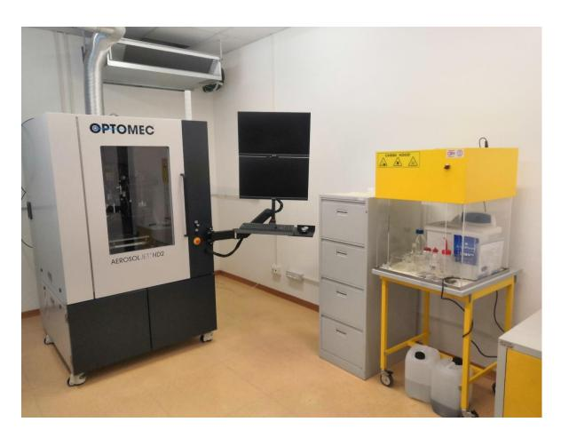
A photograph taken for the AEROSOL JET HD2 instrument provided by OPTOMEC company.
