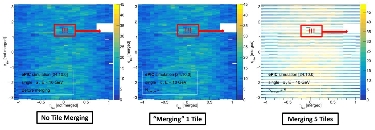
Output of merged "hits" (tiles) algorithm: (eta, phi) distribution of tiles before merging (leftmost panel) and after (right panels)
