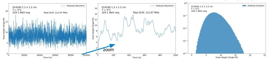
Example simulated baseline and pedestal for S14160 SiPMs at 5 °C irradiated 1e+09 1-MeV neutron equivalent dose
