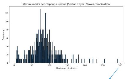
e at  $\eta$  = -1.4 (18 GeV) Max nb of pixels fired per chip
