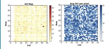
Result of w101s07 chip HV: -150V th: 100 mV External Clock source Ba133 10m data taking
