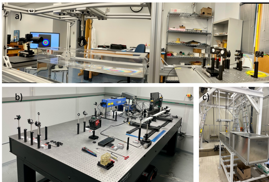
Figure 8.62: Photos of available setups developed during the hpDIRC R&D program that will be used for future QA of 3-layer lenses with laser setup at ODU (a), bars and other optics at Jefferson Lab (b) and readout chain including sensors and electronics and other hpDIRC components in hpDIRC prototype at CRT at SBU (c).
