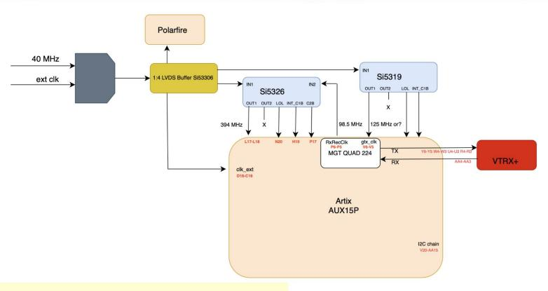
The additional Si5319 will allow us to keep flexible the frequency to be used by the VTRx+ serdes
