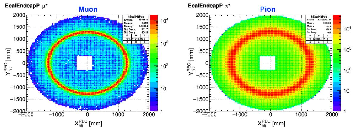
Based on muon sample (left), MIP events shows localized hits in EMCAL
