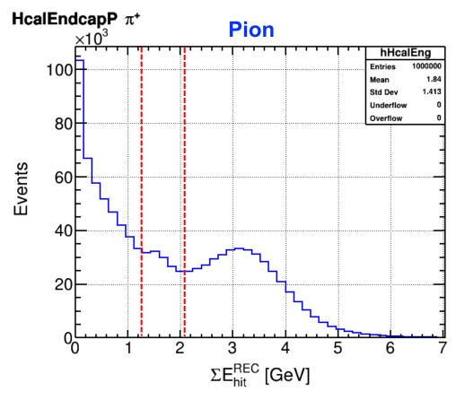
Based on muon sample (left), MIP events deposit its **energy 1.28 – 2.08 GeV in HCAL**\*Note y-axis scale difference between muon and pion samples\*
