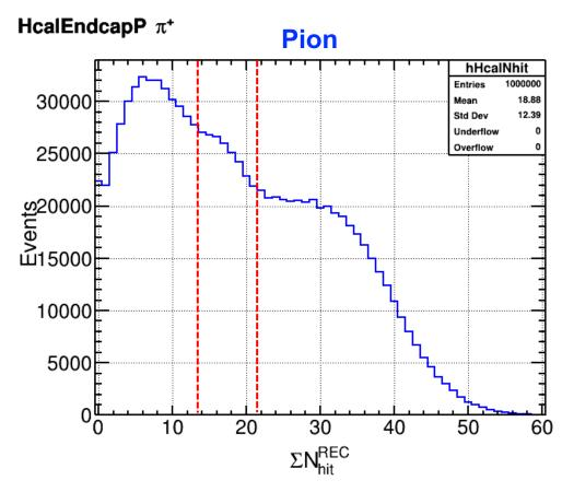
Based on muon sample (left), MIP events have **14 – 21 hits in HCAL** \*Note y-axis scale difference between muon and pion samples\*
