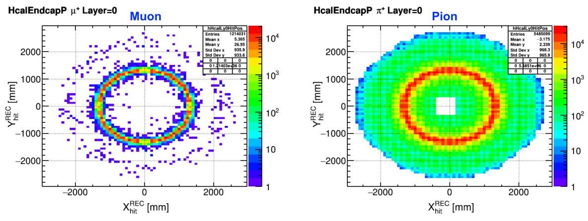
Based on muon sample (left), MIP events shows localized hits in HCAL
