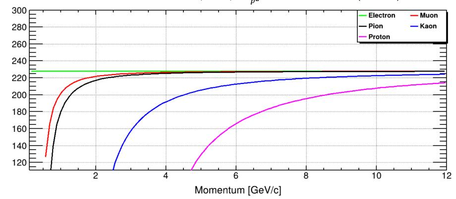
According to Chandra Chatterjee, n = 1.026 (baseline 1.019) Aerogel single photon resolution at n = 1.026 is ~ 2.4 mrad Ring (track-level) resolution ~ 0.5 mrad Given we can detect 15 photons
