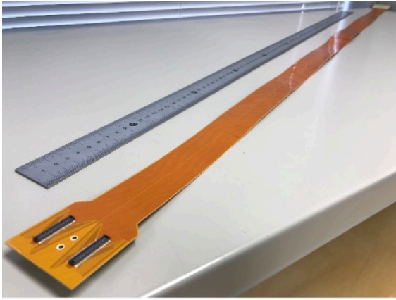
Figure 10: A photograph of the 1.11 meter long BEX cable.
