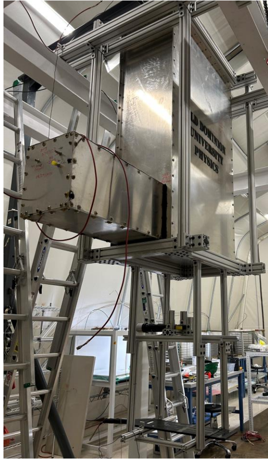
Momentum tagger installed and being tested with the scintillators
