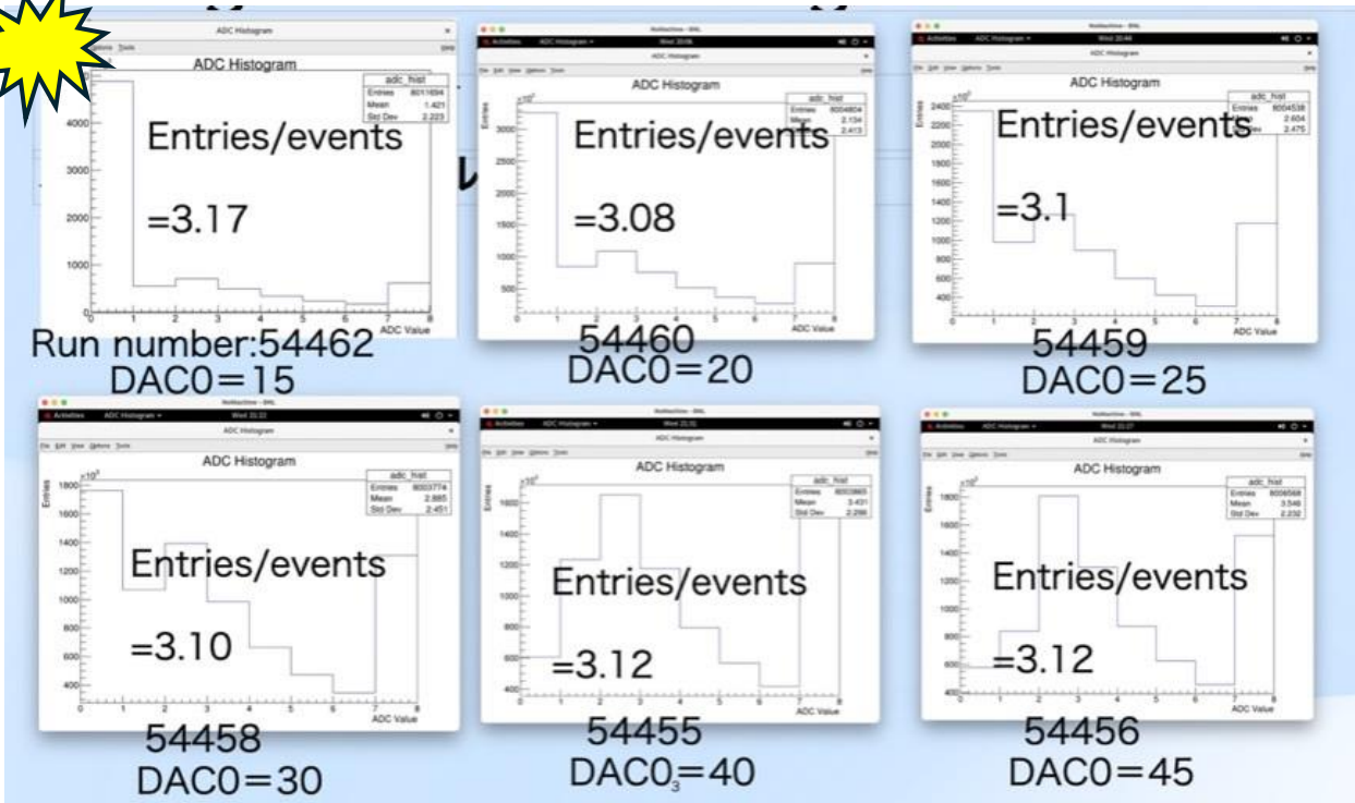
INTT's 3bits ADC Distributions for different thresholds (DAC0 value)
