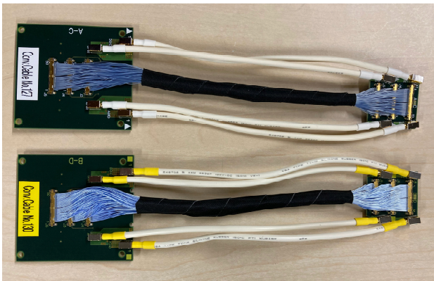
Figure 13: Conversion cable type-AC (top) type-BD (bottom). The bundles in the middle of the cable are 15 cm length \mu -coax harnesses while four white jacket cables are the power and the ground cables. The larger PC board is the connector for the BEX side and smaller one is the one for the ROC side.
