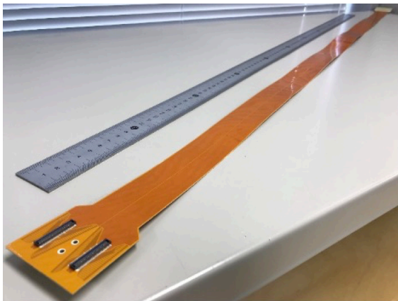
Figure 11: A photograph of the 1.11 meter long BEX cable.
