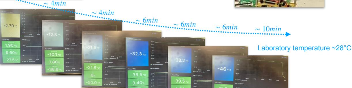
Measuring DCR on SENSL sensors breakdown voltage 24C, overvoltage 6V
