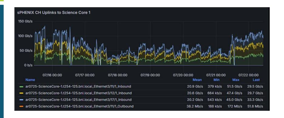
Network traffic on one of two LACP links between sPHENIX and SCDF. (Transfers to HPSS and Lustre).
