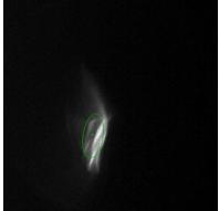
Beam on dump yag with 70-75% transmission
