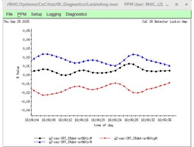
IR signal from pyro detector, bunching voltage reduced to 156 kV, close to our nominal for PCA demonstration
