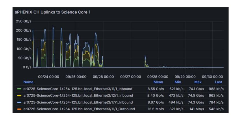
Network traffic on one of two LACP links between sPHENIX and SCDF. (Transfers to HPSS and Lustre).
