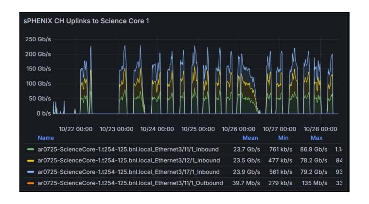
Network traffic on one of two LACP links between sPHENIX and SCDF. (Transfers to HPSS and Lustre).
