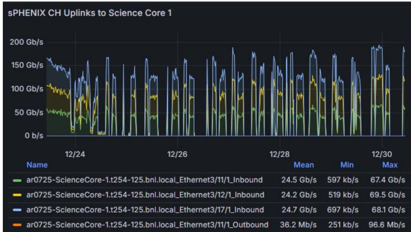
Network traffic on one of two LACP links between sPHENIX and SCDF. (Transfers to HPSS and Lustre).
