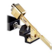
Light probe for laser delivery with 5um lens spot
