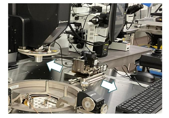
To cover full 300mm range, a custom sliding rail can be added to extend the reach of the positioner
