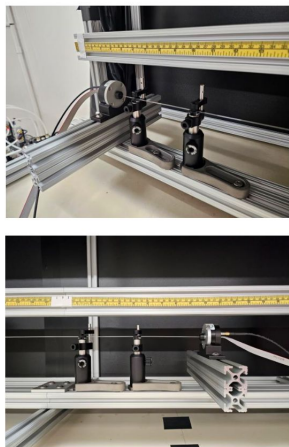
SiPM on both end S13360-1350CS
