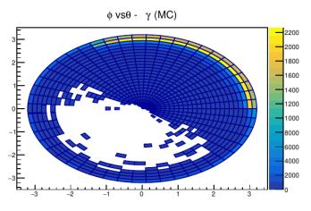
Partial detector coverage is present at MCParticles level.
