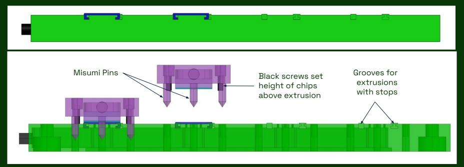
Aluminum extrusions are positioned onto plate and the vacuum is engaged. The chips are aligned in the chip tray and picked up. The locating pins on the pickup tool engage with the bushings in the gluing plate. Adjustable screws set the height of the chips above the extrusion. The pickup tools are screwed down into the gluing plate to keep them in place while the glue is curing (otherwise the vacuum hoses could make the tools tilt).
