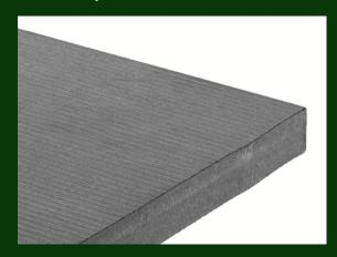
Metapor aluminum is porous to let air and moisture escape, which prevents bubbles and blemishes. These sheets must be milled to expose the pores; average pore diameter is 0.0006" with a total porosity of 15%.
