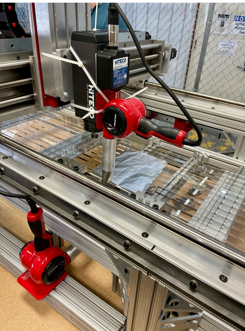
Heat guns softening glue joints between bars
