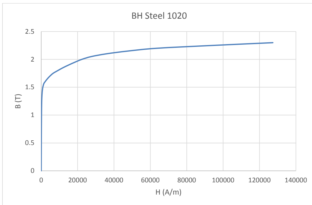
Figure 3.6 BH curve of 1020 steel
