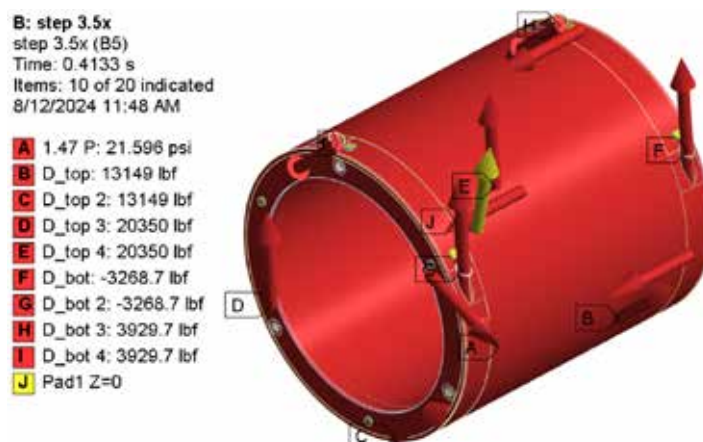
Figure 6.13 Boundary condition for Step 3.5x
