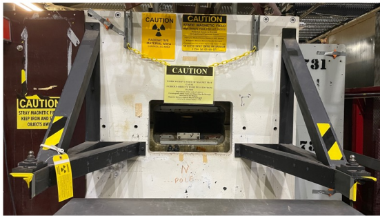
A type 18D72 2.2 Tesla dipole with a 6" gap
