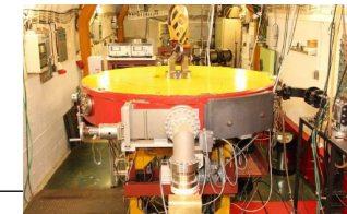
Electrons 5.5 \text{ MeV} < E_e < 16.6 \text{ MeV} ; adjust beam intensity to illumination with g rays (Co-60, 30 Gy)
