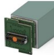
Optical coupling between the SiPM PCB and the crystal. Quality control by the other side (front)
