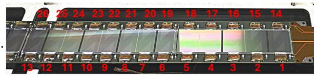
FPHX chip to ROC Data is transferred by two sets of LVDS standard output lines.
