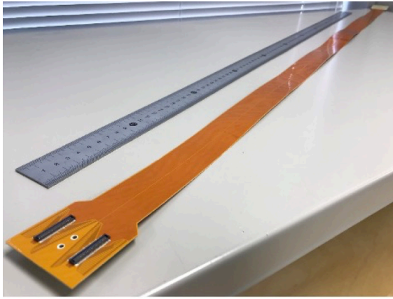
Figure 15: A photograph of the 1.11 meter long BEX cable.
